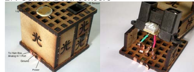
Figure 5: The GUANG BOX consists of a photocell sensor and an infrared ray sensor.
