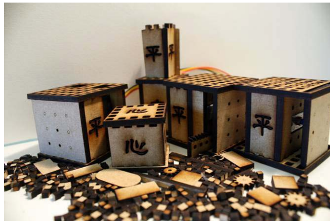
Figure 1. The TOPAOKO kit is made in laser cut hardboard embedded with circuit.
